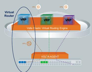
*The vAgent works in tandem with a Volta Cluster to create Virtual Routers. Up to 255 VRs can be supported on a single device.*
